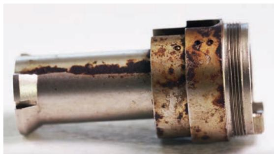
**Fig. 1:** Dental handpiece coupling with rust.
